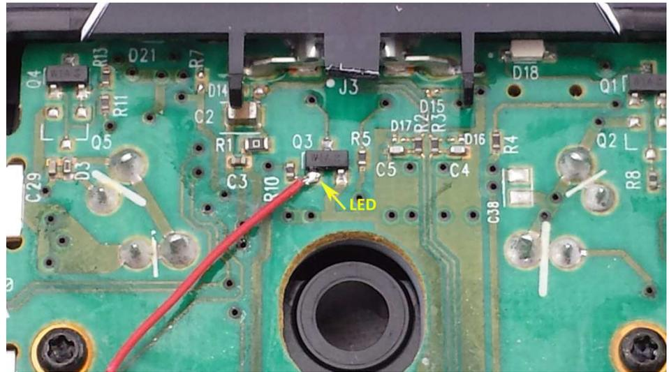
Note that for the RT and LT connections, the bottom pin of the resistor (left) and capacitor (right) are joined, so you are ok to connect the wire going over both pins like we do.
