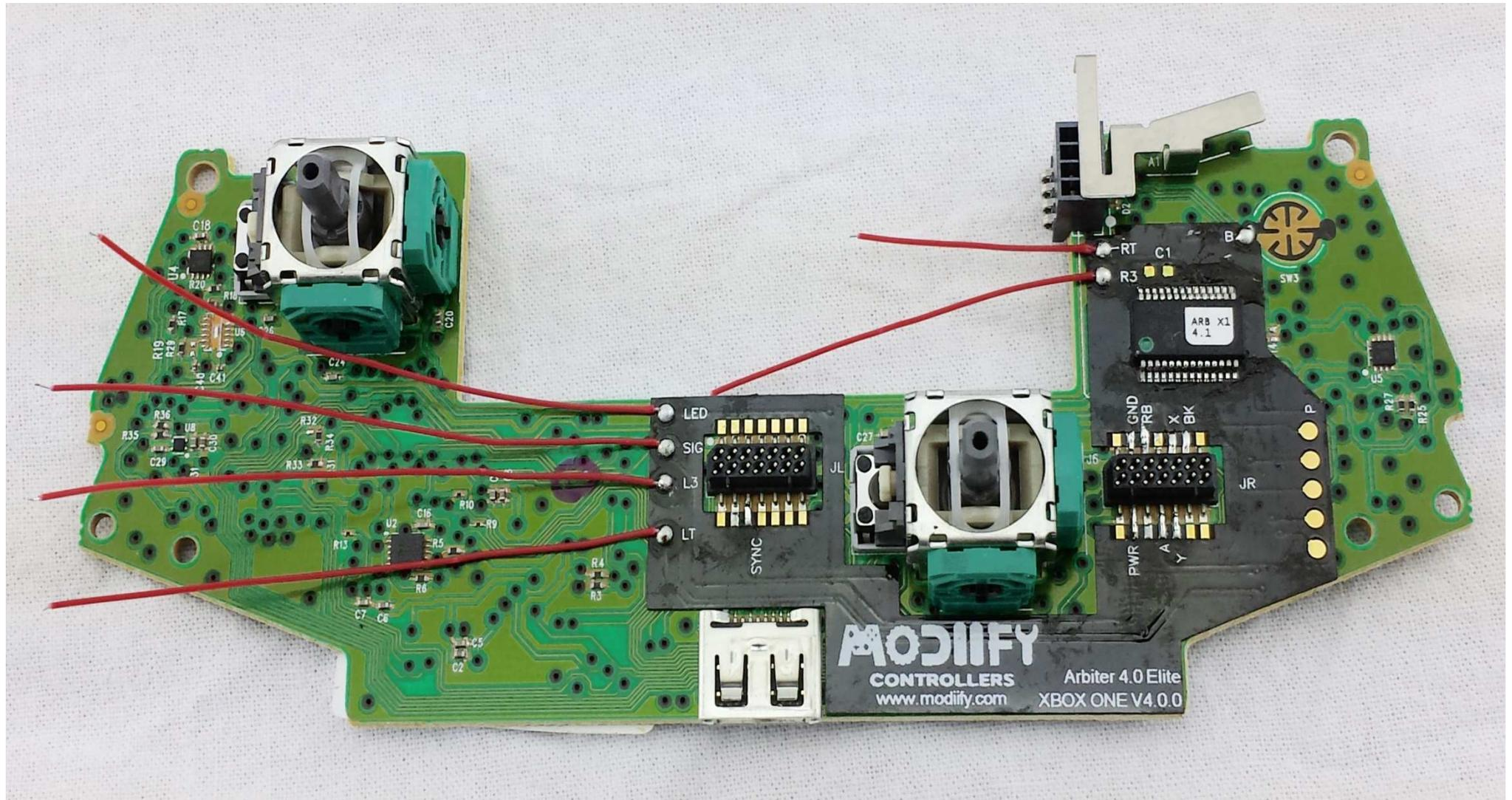
Attach the wires for the RT, R3, LED, SIG, L3 and LT pads.
