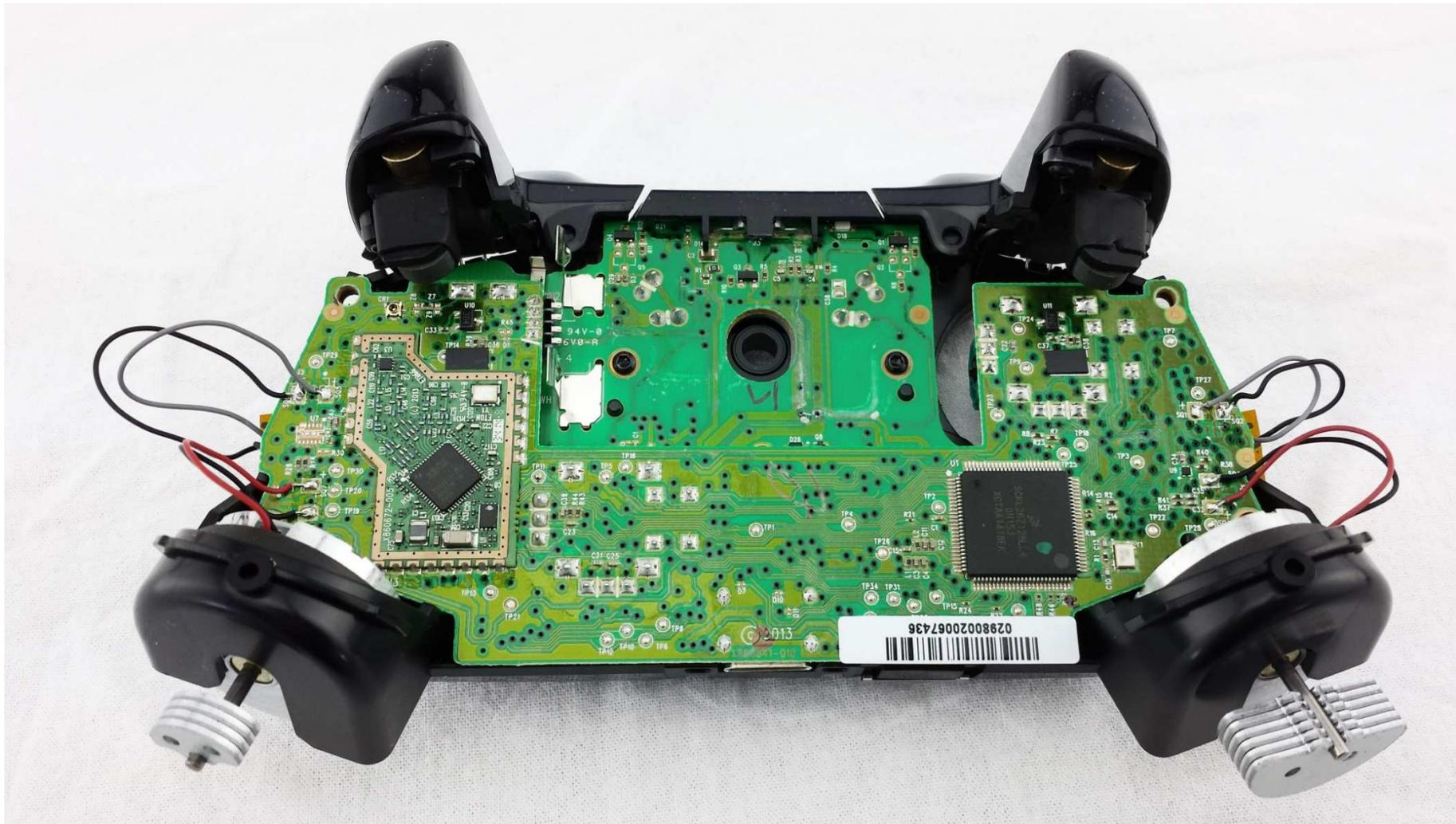
**Remove the Rumble cables from the Triggers and Rumble Motors.
